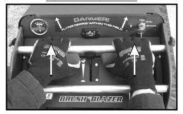
Grab the front handle bar with your fingers and the steering control handles with your thumbs. Push both steering control handles forward at the same time to move forward. Push the controls slightly to move forward slowly. Pushing harder will increase the speed of your forward movement.
